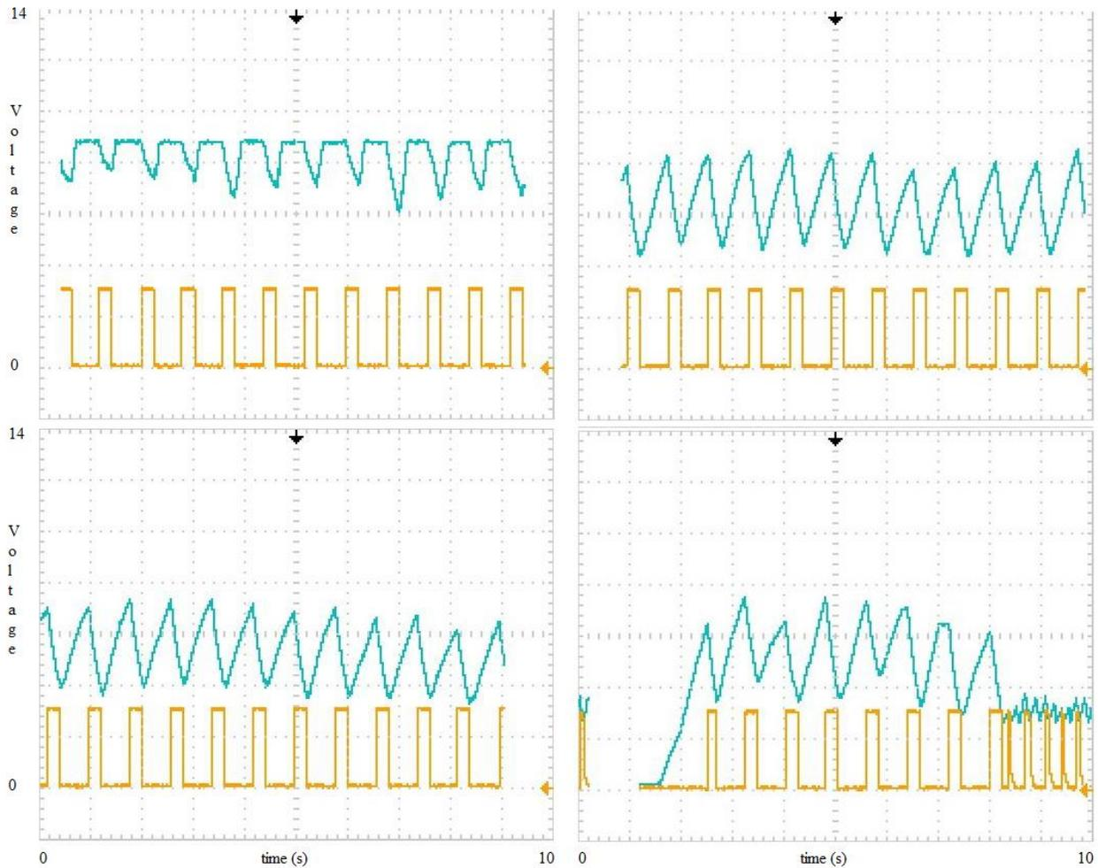
**Figure 15: WISP Power trace when computing and transmitting SQUASH packet. Blue trace is voltage and yellow trace denotes computation. WISP distance from reader, from top left to bottom right: 6", 12", 24", 30".**
